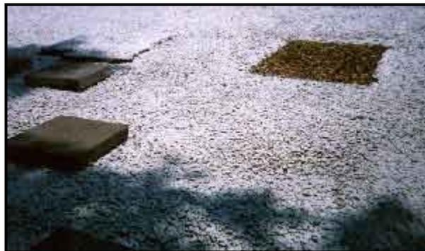
Figure 1. Uncoated patch (upper right) and coated piece (upper left) for solar reflectance samples at Tyndall Air Force Base
