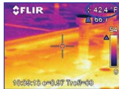
Figure 5 – Temperature of EPDM membrane.
