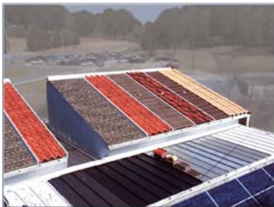
At Oak Ridge National Laboratory, cool-color roofing materials are tested with the Envelope Systems Research Apparatus.
